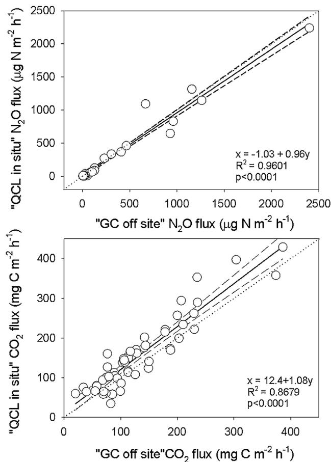
**Fig. 2.** Comparison of (a)  $\text{N}_2\text{O-N}$  ( $\mu\text{g m}^{-2} \text{h}^{-1}$ ) and (b)  $\text{CO}_2\text{-C}$  ( $\text{mg m}^{-2} \text{h}^{-1}$ ) fluxes measured from the same chambers by "QCL in situ" and "GC off site" techniques (solid line; 54 individual chamber/incubations) during field incubations. The dotted line represents a 1:1 relationship; the dashed line represents the 95% confidence interval.
