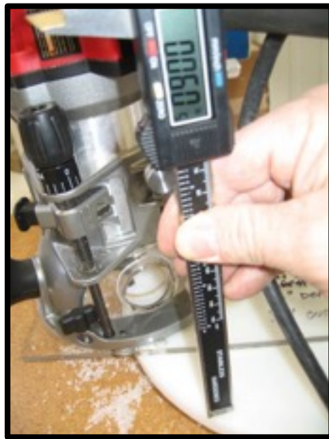
Figure 5. Lid top groove routed to 1/16" depth.
