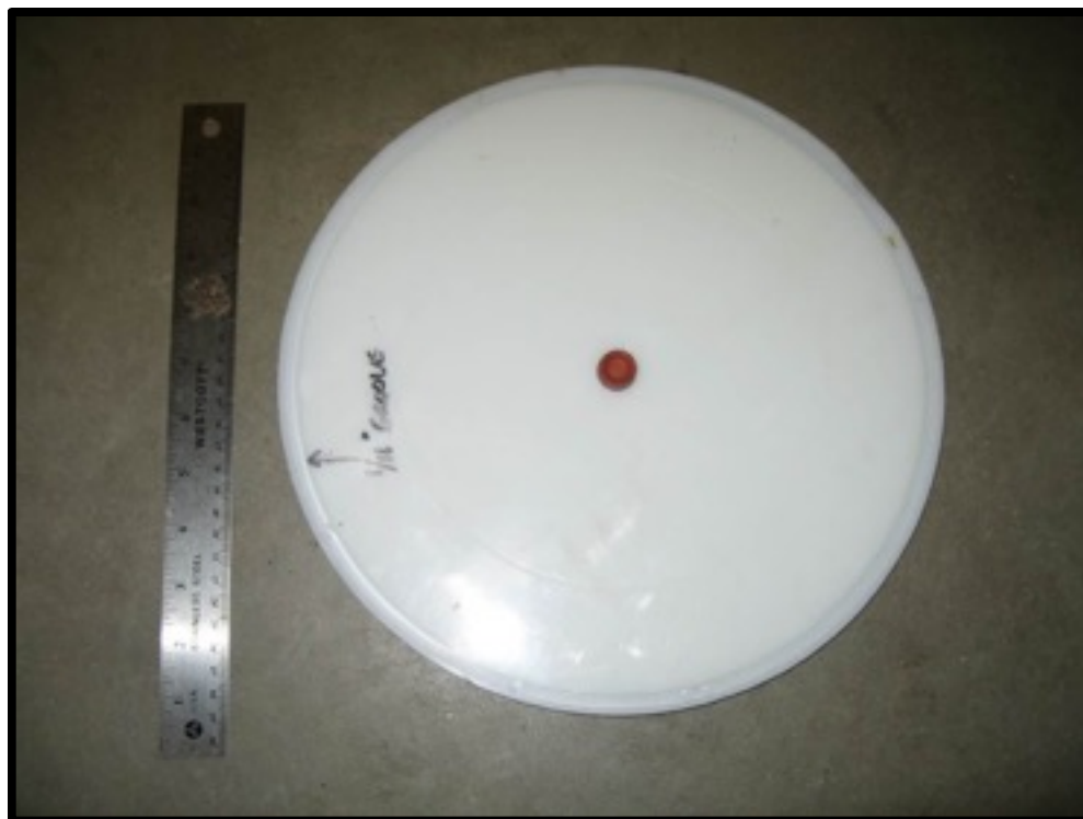
Figure 2. Lid Top with 1/4"x1/16" depth groove
