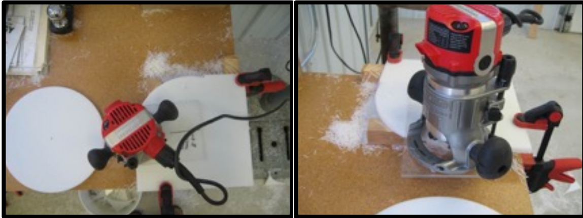
Figure 3. Routing the lid outer dimension
